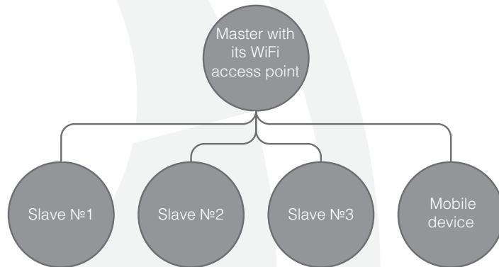
In this case the master can simultaneously handle up to 32 slave connections and the smart home system. You can also connect several master devices to the router network to enable zone-specific control.
